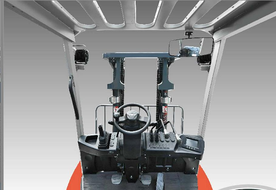
Wide view mast optimizes the blind area of operation vision and ensures comfortable and safe operation;
