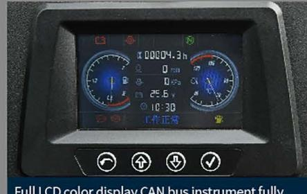
Full LCD color display CAN bus instrument fully monitors truck status; displays real-time engine and truck fault information and gives humanized reminder;
