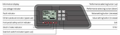
The reliable special instrument gives a complete display of the vital information, like operation status, fault detection, etc. It ensures the operator predominate the vehicle status more intuitive and convenient.
