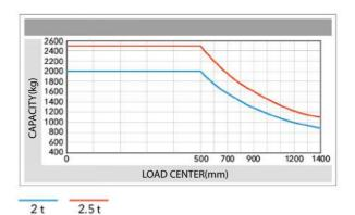
Note: The vertical axis stand for load capacity and the horizontal axis stand for load center which is calculated from the front surface of the forks to the gravity of the standard load. The standard load mean a cubic with 1000mm edge length. When mast is tilted forward, using non-standard fork or loading large goods, the load capacity will be reduced. The load capacity of standard mast at different load center can be known from this load
