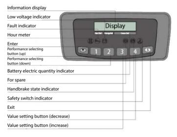
The reliable special instrument gives a complete display of the vital information, like operation status, fault detection, etc. It ensures the operator predominate the vehicle status more intuitive and convenient.
