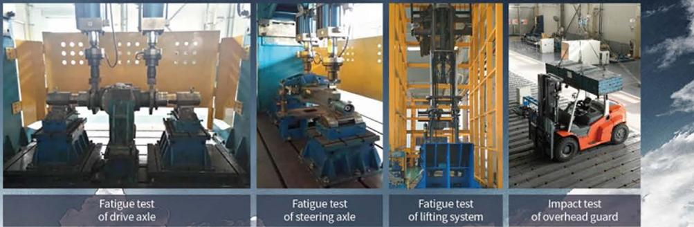
Fatigue test of drive axle
