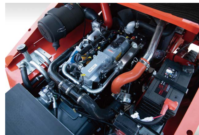
The diesel filter and engine oil filter of the engine are placed in front for easy daily maintenance
